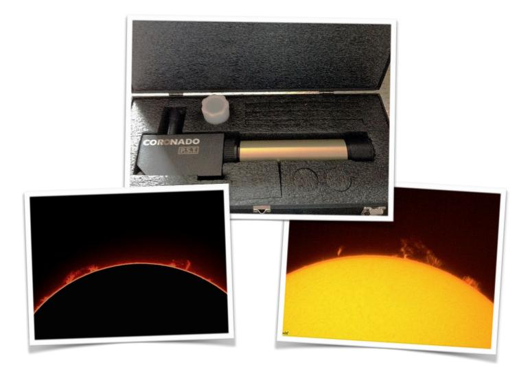
How I image with the Coronado PST Hydrogen Alpha + Canon 350D Single exposures (no Stacking)
