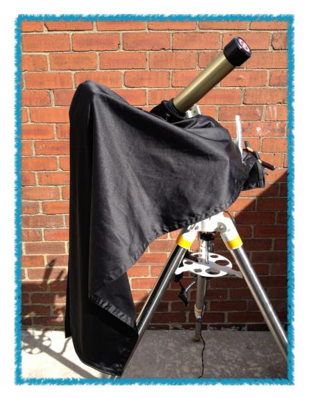
and wrap as much as possible around the camera area and this gives you a higher contrast view without any sunlight creeping in, this really does help especially on wispy prominences and filaments.
