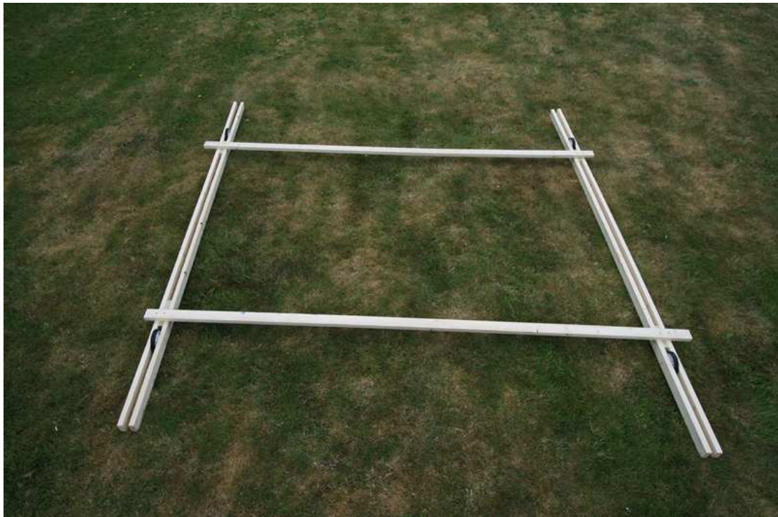
Figure 38 – Prepare for test of runners (two temporary cross braces shown)
