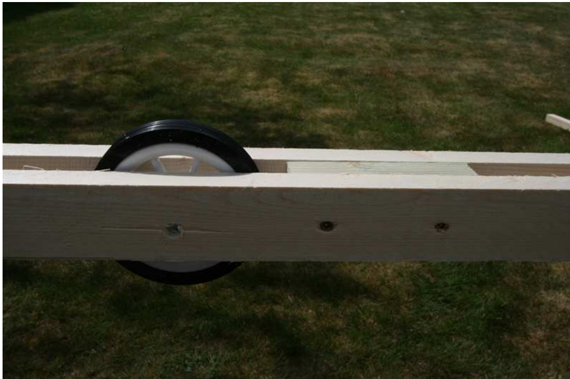
Figure 34 – Close up of captive roof runner wheel
