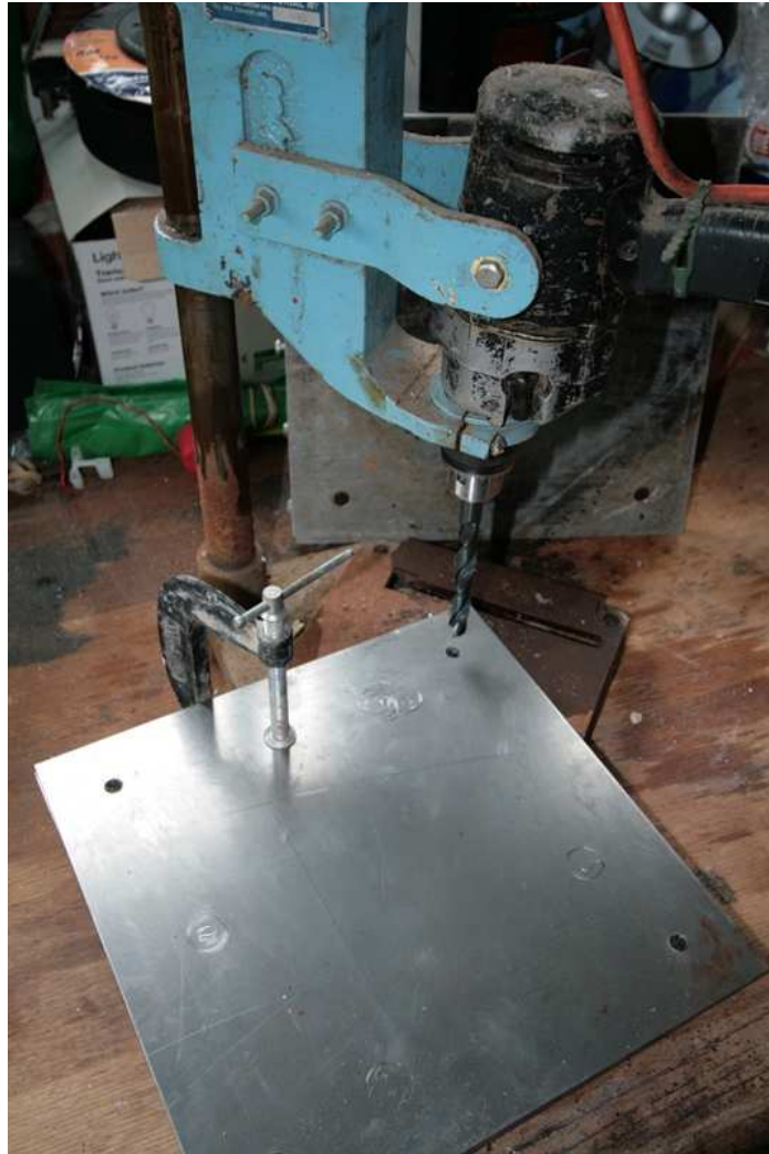
Figure 77 – Drill clearance holes for the 12mm studding in both plates
