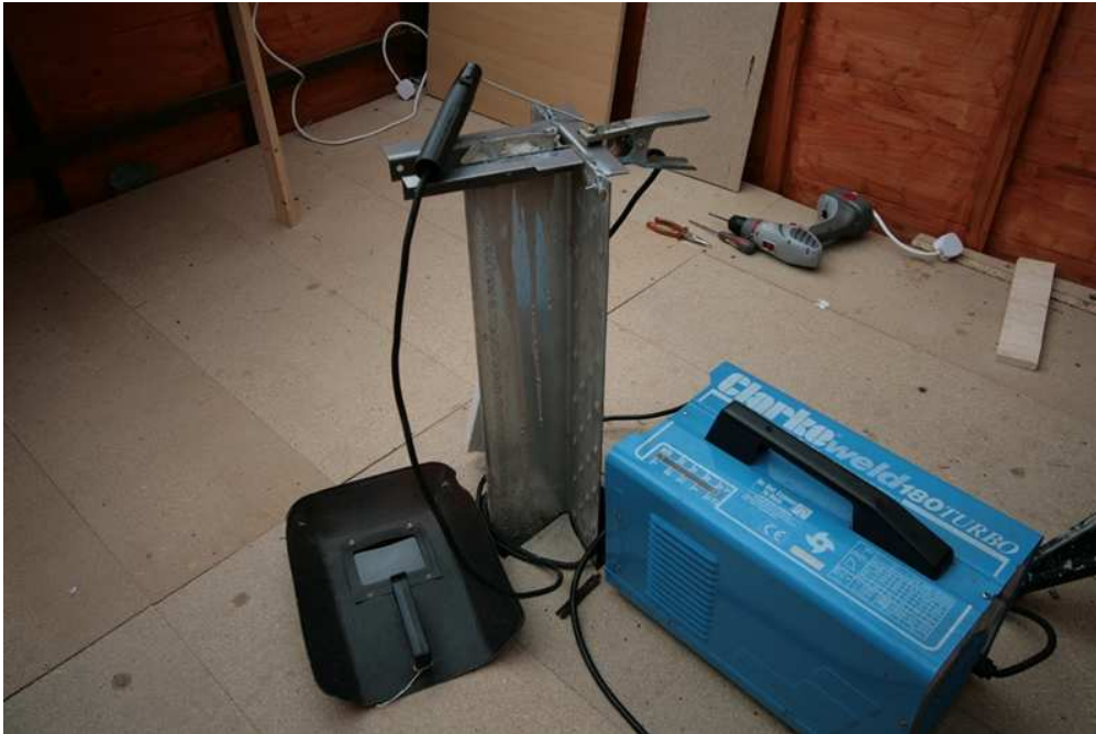
Figure 81 – Prepare to arc weld the bottom plate to the pier
