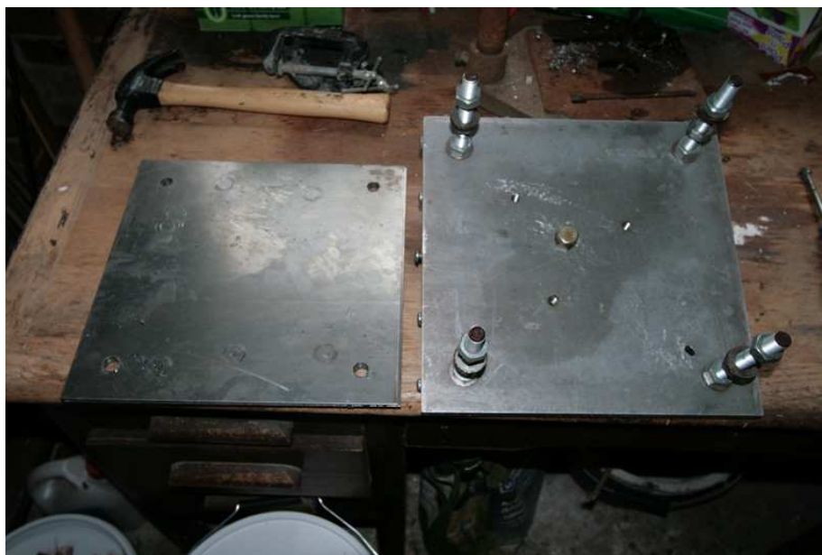
Figure 78 - Prepare pier head for Meade superwedge support (2)
