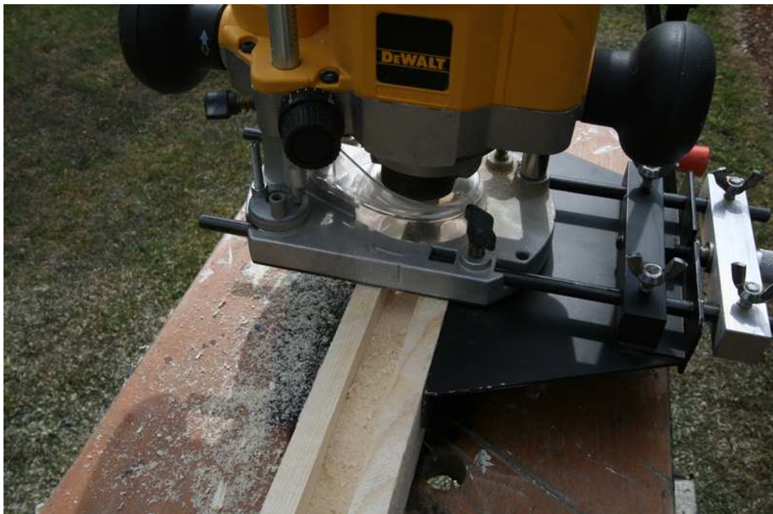
Figure 22 – Cutting out a 20mm channel for the roof wheels to run in
