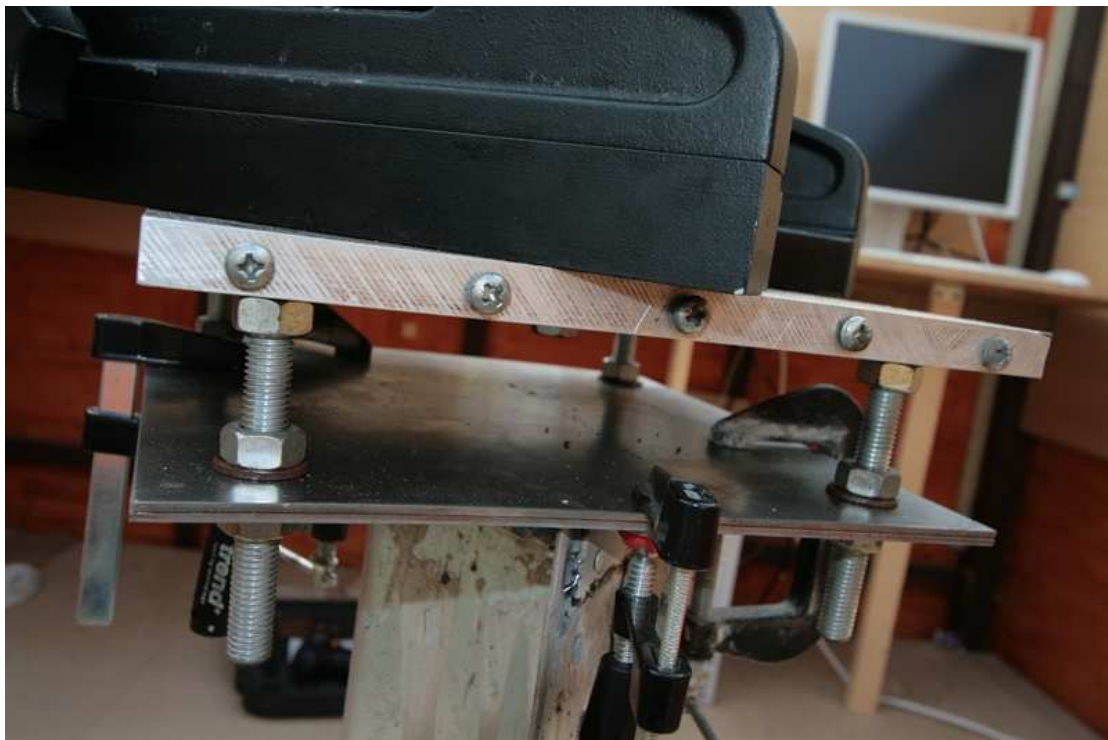
Figure 82 – Bottom plate welded in place and locked to top plate
