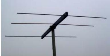
Figure 5.1 3 Element Yagi
