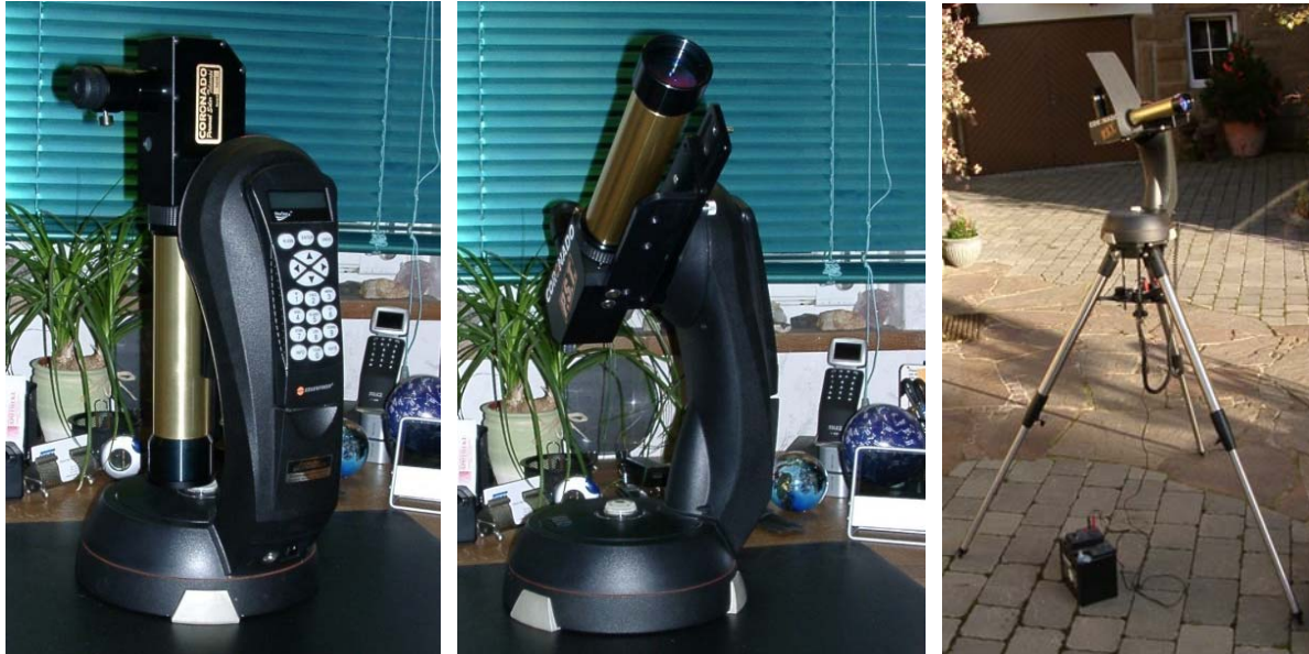
Here you can see the PST attached to the N5i mount and outside on the tripod
