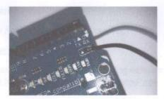
PPS marks the edge of the precise second transition from the GPS and is used here as an interrupt to enable UTC to be determined to an accuracy of a few microseconds within the server.
